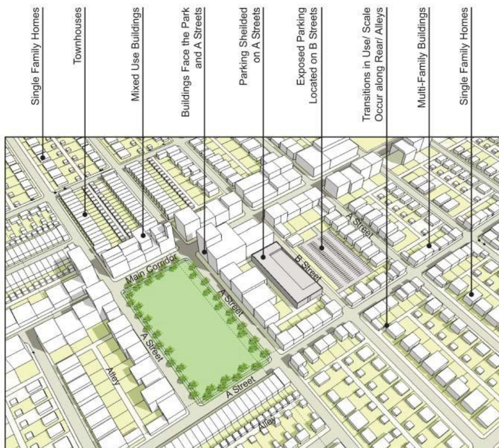
Illustration of transition of uses, scale, and massing. Note the use of roads and alleys in the transition between varying intensities.
